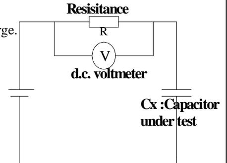
Figure4.Circuit for leakage current method
