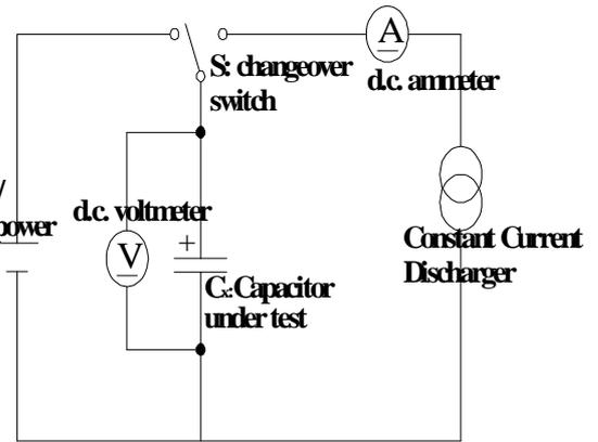
Figure1. Circuit for constant current discharge method
