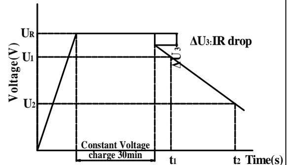
Figure2. Curve for charge-discharge
