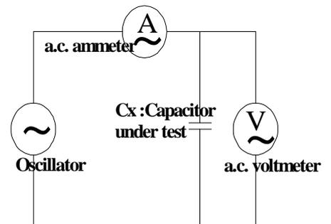
Figure3. Circuit for AC internal resistance method
