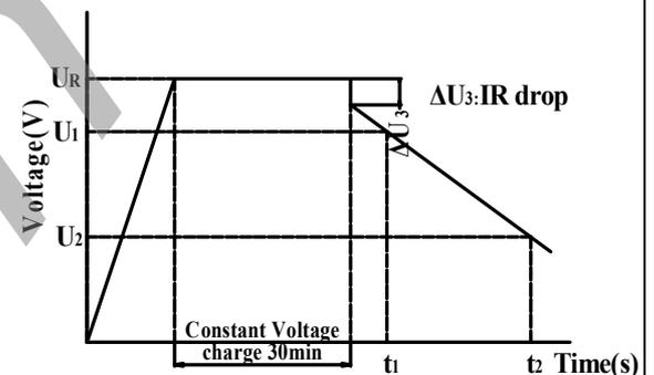
Figure2. Curve for charge-discharge
