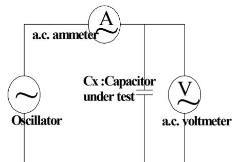
Figure3. Circuit for AC internal resistance method
